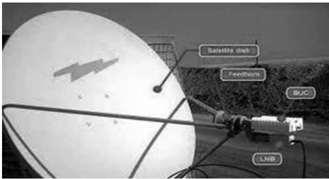
Fig: Satellite remote dish antenna with necessary equipments
