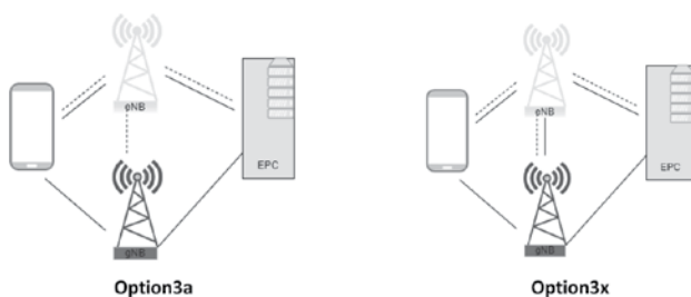
Fig. 6: Option3a and 3x NSA, EPC with NR and LTE.
