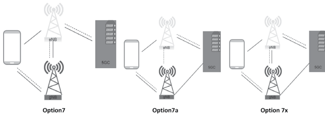
Fig. 9: Option7 NSA, 5GC with NR and LTE.
