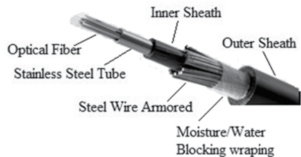
Fig. 1: Structure of Direct Buried Cable [ITU-T L.110].
