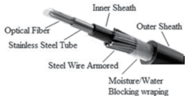
Fig. 1: Structure of Direct Buried Cable [ITU-T L.110].
